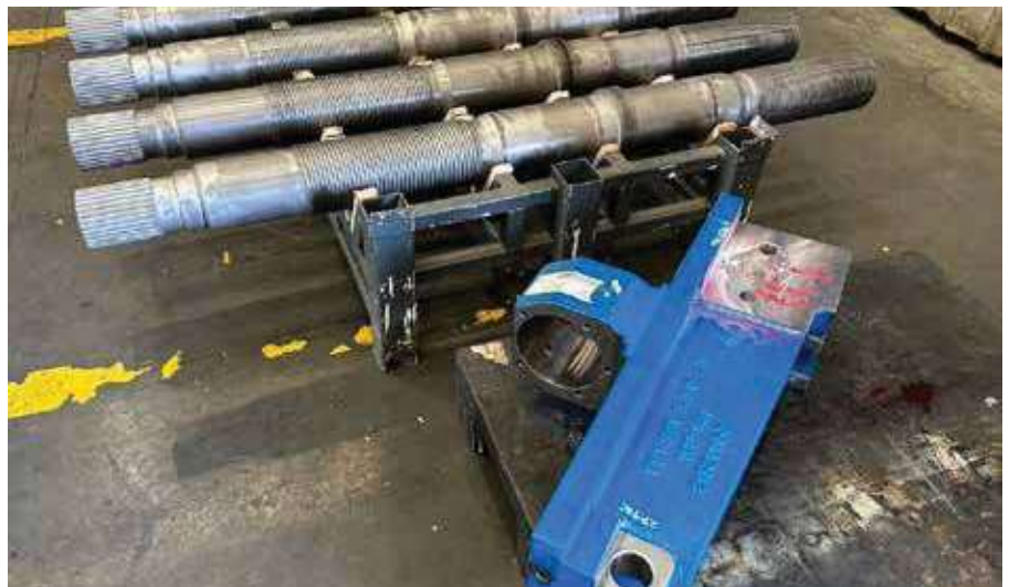
Fig. 1 • Machine components made of cast iron, type GJS-400-15 (EN 1563), which should be repaired by local deposition welding. (Picture: Alpha Laser Southeast Asia Co., Ltd.)
