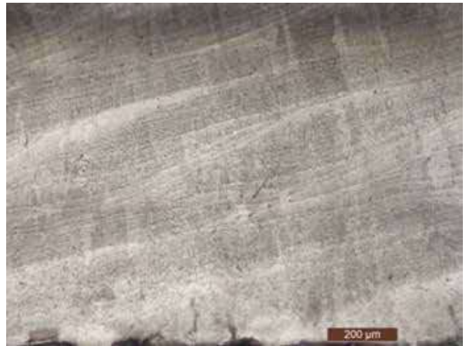
Fig. 7 • Pure weld metal of the welded work-plate (Picture: Alpha Laser Southeast Asia Co., Ltd.)
