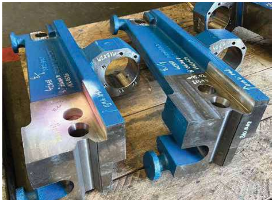
Fig. 2 • Machine components made of cast iron, type GJS-400-15 (EN 1563), which should be repaired by local deposition welding. (Picture: Alpha Laser Southeast Asia Co., Ltd.)
