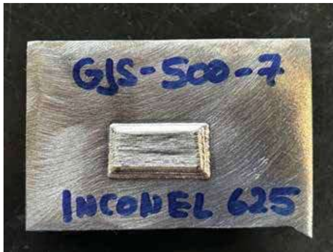
Fig. 4 • Work sample with three-layer pulsed laser deposition welding. (Picture: Alpha Laser Southeast Asia Co., Ltd.)
