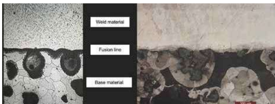
Fig. 5 • left: Micrograph of GJS-400-15 cast material (carbon content 3.25 to 3.70%) with an “alien” deposition welding performed by conventional manual arc welding with a Ni-Fe filler metal; right: Micrograph of EN-GJS-500-7 ductile iron material (carbon content 3.40 to 3.60%) with an “alien” deposition welding performed by the “energy of light”, by pulsed laser beam welding. (Picture: Alpha Laser Southeast Asia Co., Ltd.)
