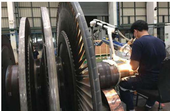
Fig. 5 • On-site welding on the turbine rotor.
