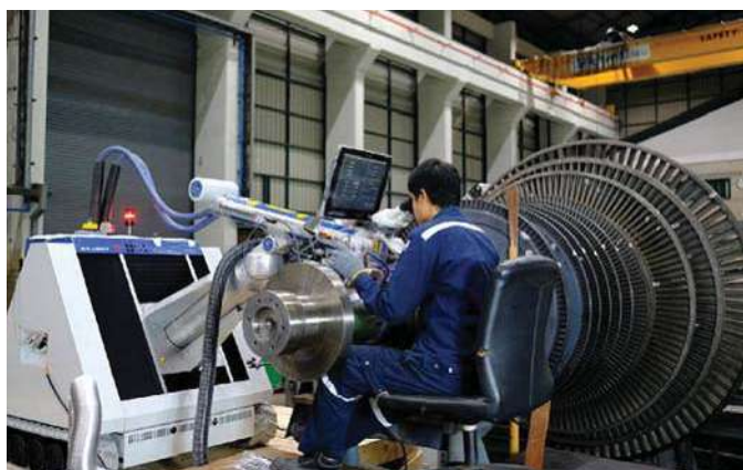
Fig. 2 • The Nd:YAG pulsed laser welding machine "900W ALFlak fibre" from the German manufacturer Alpha Laser in the welding application at the turbine rotor in Thailand.
