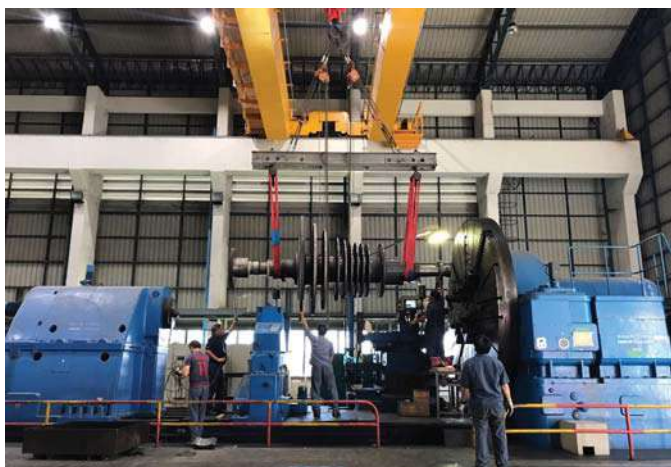
Fig. 1 • Placing the turbine rotor on the head lathe for mechanical pre-machining of the damaged surfaces.
