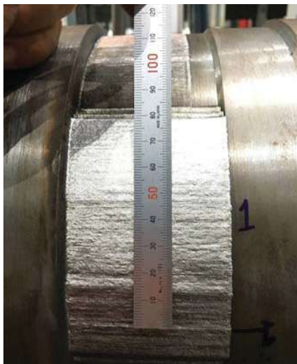
Fig. 6 • Layer structure of the pulsed laser beam repair welding.
