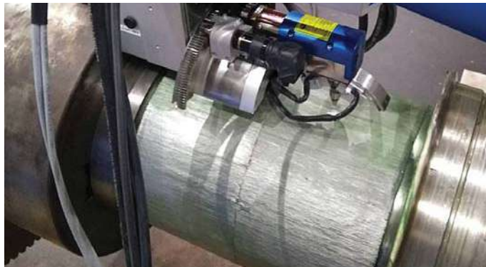
Fig. 7 • The finished pulsed laser beam weld during the final stress check.
