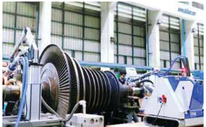
Fig. 11 • Simultaneous pulsed laser beam deposition welding on both rotor shaft ends.
