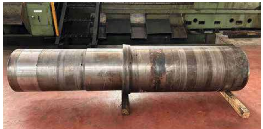
Fig. 7 • Mechanically prepared bearing seat shaft.
