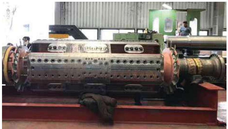
Fig. 12 • Squirrel-cage rotor before deposition welding.
