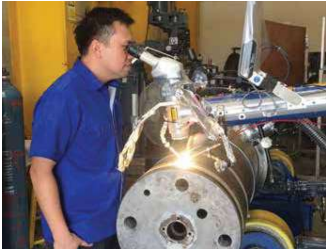
Fig. 8 • Temporary monitoring of the weld seam quality through the eyepiece of the pulsed laser beam welding machine.
