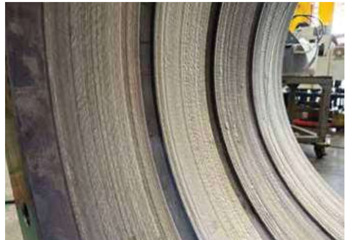
Fig. 5 • Completely welded bearing seats.
