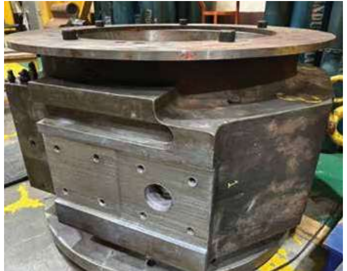
Fig. 9 • Shock absorber housing with reference surface.
