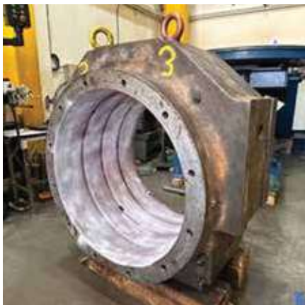
Fig. 6 • Shock absorber housing after dye penetrant testing.
