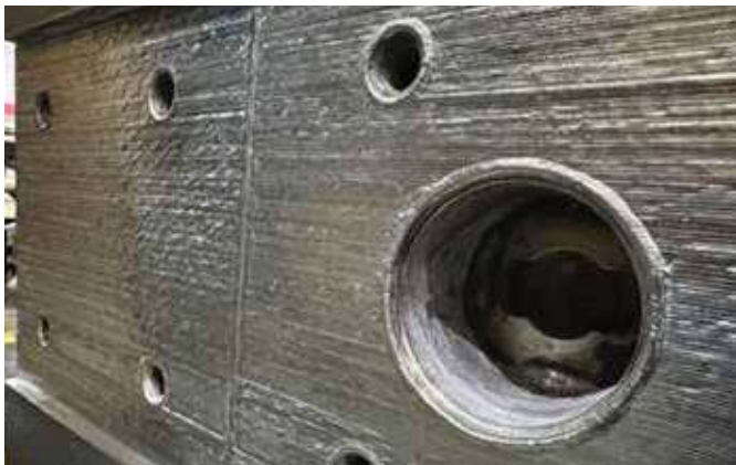
Fig. 10 • Detailed view of the reference surface welded by pulsed laser beam welding.
