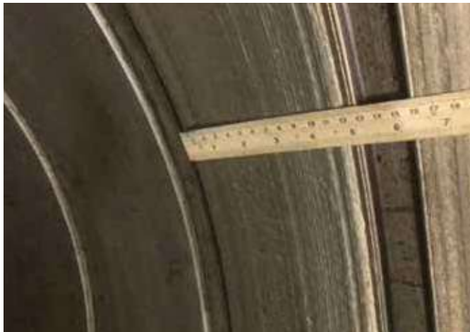
Fig. 4 • Partially finished welded bearing seat.
