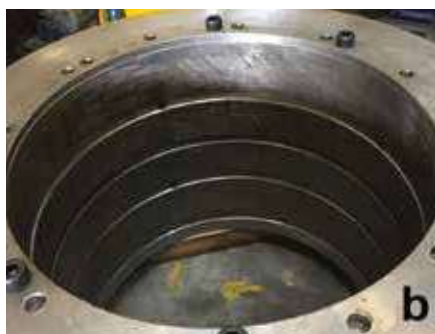
Fig. 1 • Shock absorber housing with mechanically machined bearing seat surfaces prepared for welding. (Pictures: Alpha Laser Southeast Asia Co., Ltd.)
