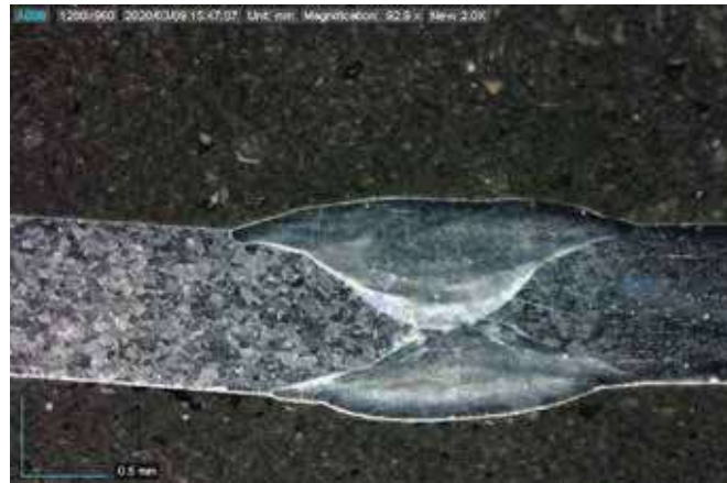
Fig. 5: Macrosection of a successful position-counterposition joint weld with no significant heat-affected area of the base metal "Inconel 625", test piece thickness: 0.54 mm. (© DSI Laser Service (Thailand))
