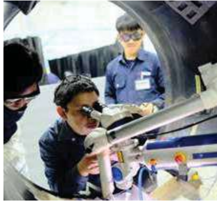
Fig. 9: Repair welding by pulsed laser on a conical exhaust gas jacket made of "Inconel 625" and constructed using honeycomb technology. (© DSI Laser Service (Thailand))
