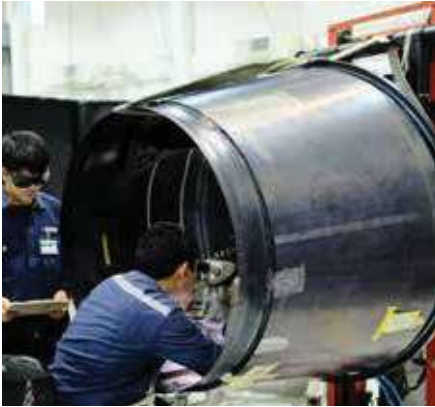
Fig. 9: Repair welding by pulsed laser on a conical exhaust gas jacket made of "Inconel 625" and constructed using honeycomb technology. (© DSI Laser Service (Thailand))
