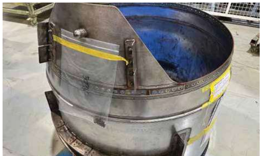
Fig. 3: Conical honeycomb exhaust jacket made of “Inconel 625”. (© DSI Laser Service (Thailand))
