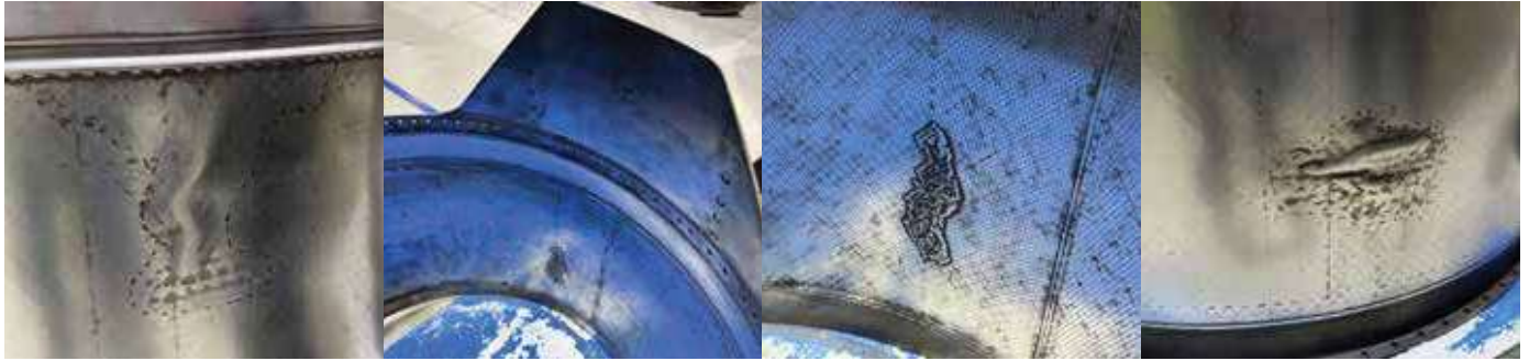
Fig. 7: Examples of areas in need of repair by pulsed laser: dented outer shell (left); inner shell previously repaired by TIG or MIG welding (rest). (© DSI Laser Service (Thailand))
