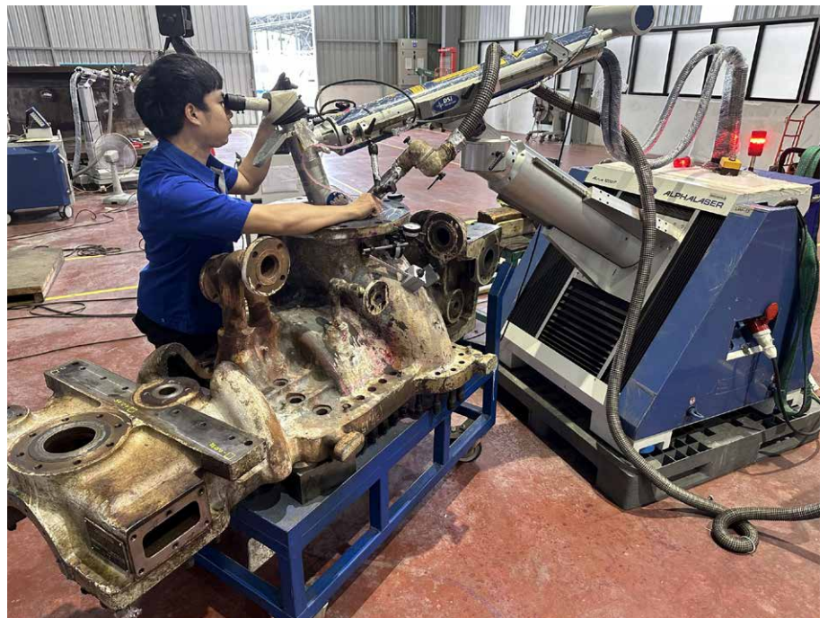
Fig. 6: Structure of component and fiber laser machine during pulsed laser beam welding (© DSI-Thailand)
