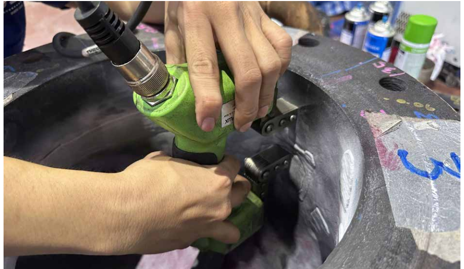
Fig. 7: Various methods were used for the final quality control, the picture shows the magnetic particle testing at the gas outlet nozzle (© DSI-Thailand)
