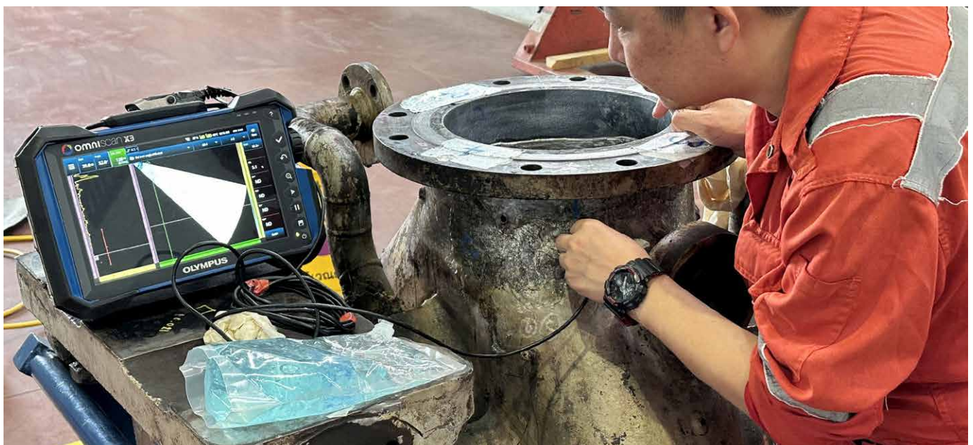
Fig. 9: Ultrasonic testing at the gas outlet nozzle (© DSI-Thailand)
