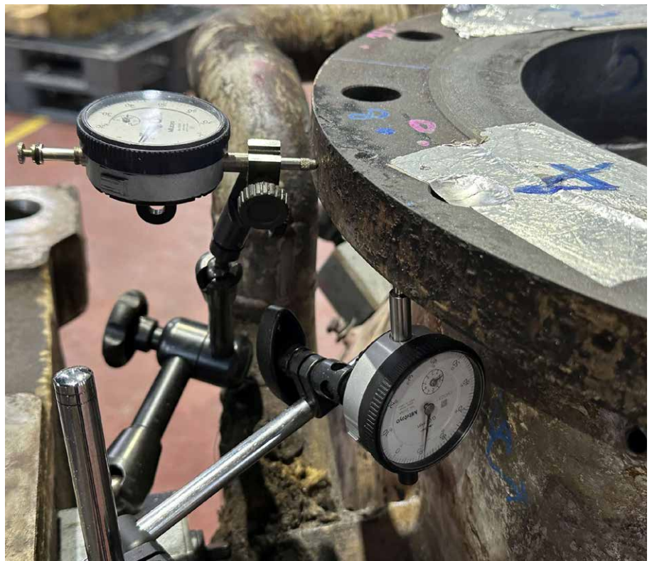
Fig. 4: Measuring setup for checking any welding distortion (© DSI-Thailand)
