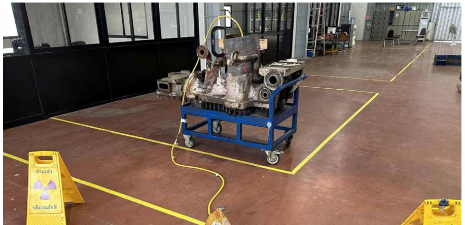
Fig. 8: Radiographic testing at the gas outlet nozzle (© DSI-Thailand)
