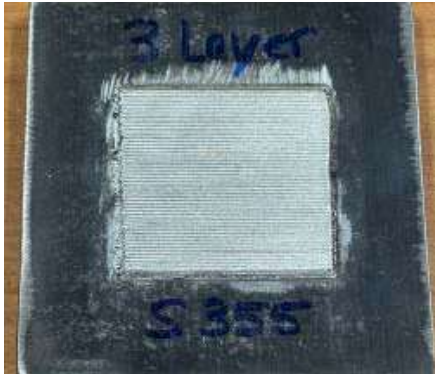
Fig. 14: Three-layer pulsed laser beam welding (© DSI-Thailand)
