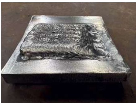
Fig. 4: Three-layer manual metal arc welding (© DSI-Thailand)
