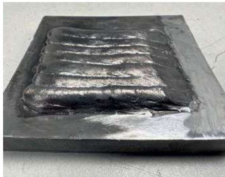
Fig. 8: Three-layer MAG welding (© DSI-Thailand)
