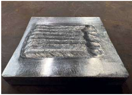
Fig. 2: Single-layer manual metal arc welding (© DSI-Thailand)
