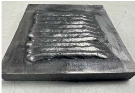
Fig. 6: Single-layer MAG welding (© DSI-Thailand)
