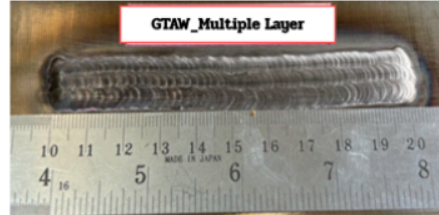
Figure 8 : GTAW Multiple layer (GTAW3L) Weld Bead
