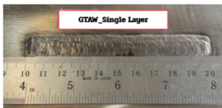
Figure 7 : GTAW Single Layer (GTAW1L) Weld Bead
