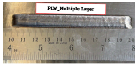
Figure 6 : PLW Multiple layer (PLW3L) Weld Bead
