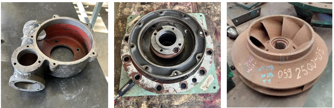
Fig 1: Representative nodular cast iron components commonly used in industrial applications:
